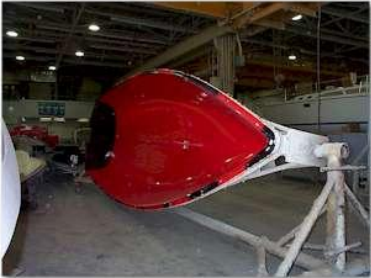
Hull mold of a Catalina 22 MkII.
